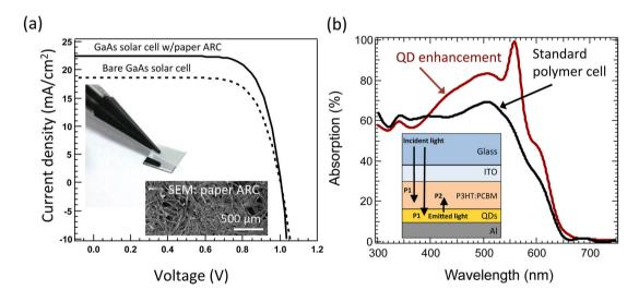
*Figure 3.* (a) Paper-based antireflection coating (ARC) leads to significant current enhancements and improved solar cell efficiencies. (b) Quantum dots (QDs) can act as scatterers to increase the absorption in thin-film solar cells. (Adapted from Xu and Munday,<sup>4</sup> and Callahan, Munday, and Atwater.<sup>5</sup>) SEM: Scanning electron microscopy (image). GaAs: Gallium arsenide. P1, P2: Photons. ITO: Indium tin oxide. P3HT:PCBM: Polymer blend.
