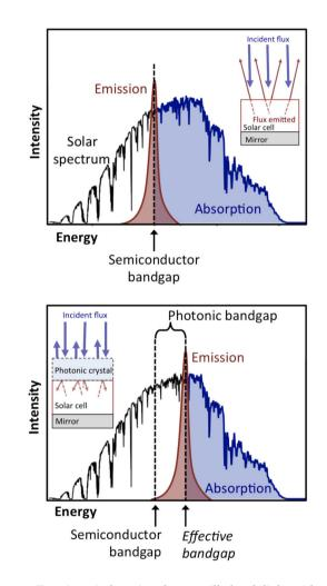
**Figure 1.** Top: A typical semiconductor will absorb light with energy above the bandgap and recombining carriers will yield emission of photons near the semiconductor bandgap. Bottom: A photonic crystal will block the flow of light both into and out of the semiconductor, resulting in the appearance of a semiconductor with a new effective bandgap.
